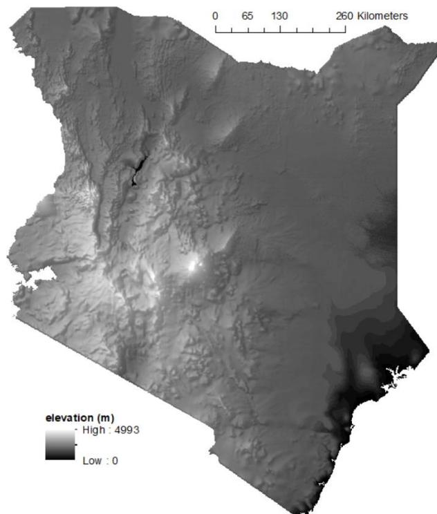
Figure 2: Digital elevation model derived from the SRTM used (whiter cell means higher altitude).
